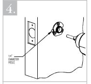
Drill a 1/4" diameter hole through both sides of the door.
