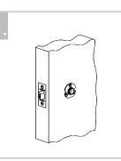
After completing the latch and backplate installation, a hole for the privacy button needs to be drilled.
